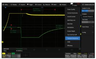
The power analysis tool can evaluate II different power supply or power device parameters such as power quality, inrush current and switching loss.
