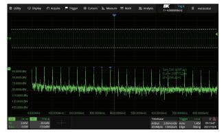
The math function provides a formula editor and various operations including an FFT with maximum memory depth of 2 Mpts. Two operations can be displayed simultaneously.
