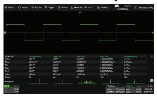
50+ different parameters are readily available with statistics displayed nominally and as a histogram. Measurements can be acquired from function, reference and history waveforms.
