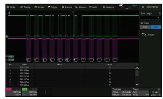
Serial bus decode supports I<sup>2</sup>C, SPI, UART, CAN, and LIN protocols. Information is displayed in tabular form.
