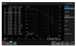
The Bode plot feature evaluates the amplitude and phase of a system with respect to frequency. Samples acquired are displayed in a graphical and tabular form.
