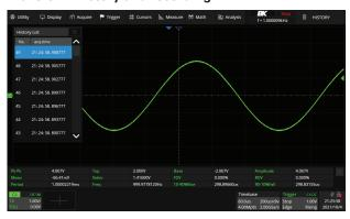
Segmented memory captures important segments of signals without wasting memory on the dead time. The history function can store up to 90,000 triggered waveforms.
