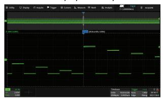
The oscilloscope's exceptionally deep memory allows you to capture waveform details over extended time intervals and at high sampling rates, then zoom into the signal for further analysis.
