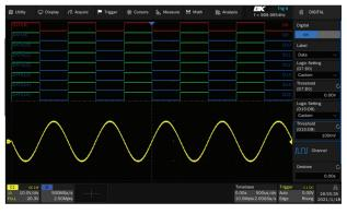
The MSO feature adds 16 digital channels allowing the acquisition and triggering of mixed signal waveforms.
