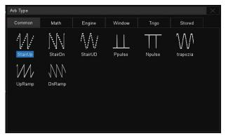
The built-in DDS waveform generator outputs waveforms with maximum frequencies of 50 MHz and  $\pm 3$  V amplitude. Sine, square, ramp, pulse, noise, DC and arbitrary waveforms are available.
