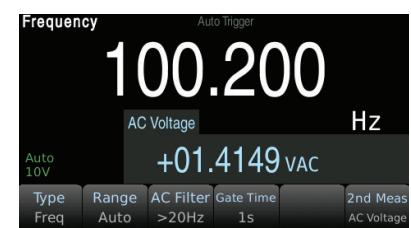
Simultaneously display multiple measurements such as frequency and AC voltage.
