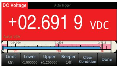
Set upper and lower limit levels with PASS/FAIL counter and indicators.
