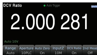
Displays the ratio between two separate DC voltage measurements within  $\pm 12$  Volts. This function is useful to quickly verify the difference between input and output magnitudes of low voltage circuits.
