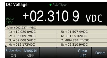
Use probe hold mode to quickly compare a series of readings. Stable readings are captured and added to a list of up to eight measurements.
