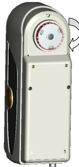
Figure 11 Turn the Measuring Aperture Clockwise About 20 Degrees
