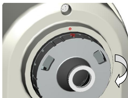
Figure 13 Turn the Extended Measuring Aperture Clockwise About 20 Degrees
