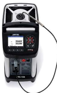
Adjust the internal reference sensor to give the same readings as the external reference sensor by performing a Self Calibration. After the Self Calibration the calibrator can be used without the external reference sensor. Regular Self Calibration is needed to ensure the accuracy. The Self Calibration is simple and fast to perform following the steps in the reference manual.
