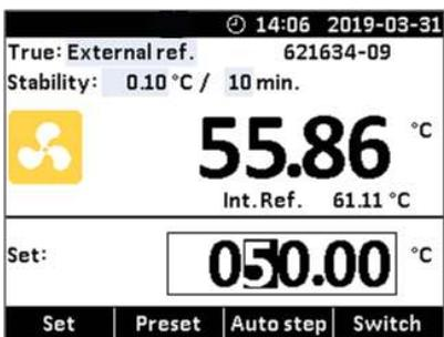
The fastest and simplest way of starting the calibrator. Simply press SET and type in the desired temperature, and off you go.
