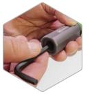
Tamper-proof internal adjustment. No external adjustment scale—must be preset using a torque analyzer.
