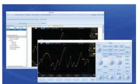
PC software is provided (free download at www.bkprecision.com) for seamless integration between the oscilloscope and PC. Capture and transfer waveforms, screen images, setups and measurement results to a Windows PC via the USB device port on the back of the instrument. A USB host port on the front allows for quick and easy screen saving.
