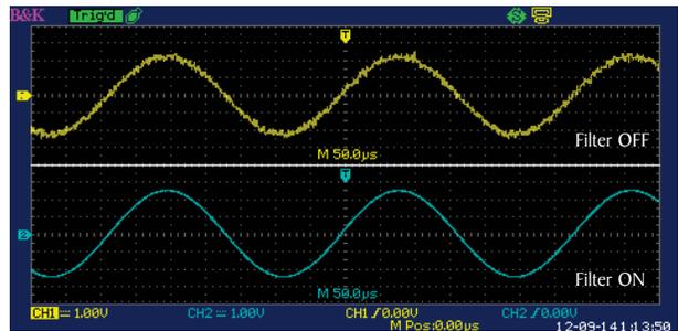
Filter out unwanted signal components such as various types of noise with built-in digital filters. Choose from Low-Pass, High-Pass, Band-Pass, and Band-Stop filters.
