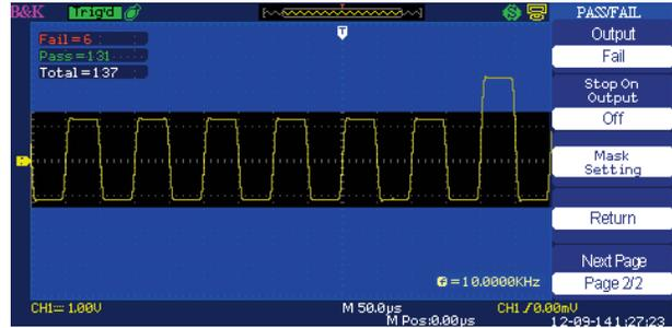
Generate user-defined pass/fail limits to quickly identify go/no go test results.
