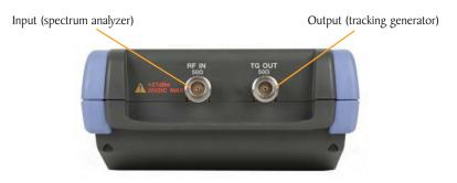
Tracking generators are ideal for tuning filters, determining the usable frequency range of amplifiers and attenuators and aligning receiver IF stages.
