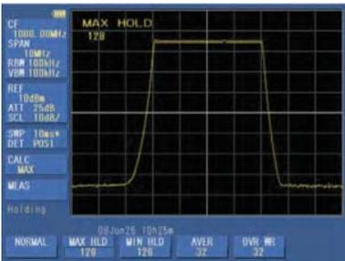
**Min hold:** At each displayed frequency, the currently-measured value is compared to the previously-measured value and the smaller one is retained and displayed.
