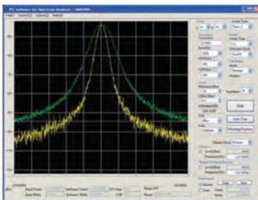
The 2650A series includes easy-to-use software for documentation and further analysis of your measurements. Connect the analyzer via USB cable to your PC, configure the analyzer remotely, then download measurement data and instrument settings for storage and further analysis.
