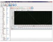
Generate, edit, and upload arbitrary waveforms to the scope using the intuitive Comsoft PC software.
