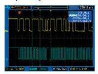
Beneficial for applications such as I<sup>'</sup>C serial data streams, deep memory lets you capture waveforms in high resolution while maintaining a high sample rate over a longer period of time. Up to 2.4 Mpts of memory can be captured in as fast as 5 seconds\* using binary transfer through the LAN or USB interface.
