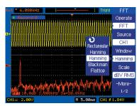
Display and measure the input signal's frequency spectrum. Select one of the 5 FFT windows: Rectangular, Hanning, Hamming, Blackman, and Flattop. Use cursors to measure the spectral component's magnitude and frequency.
