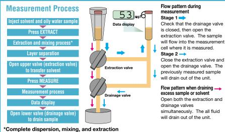
"Complete dispersion, mixing, and extraction The extraction tank uses HORIBA's specially designed agitator blades. Pushing the EXTRACT button initiates a powerful rotary dispersion and mixing action.
