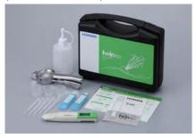
Accessories included: Standard solution for crops (300ppm & 5000ppm) (14mL), 2 CR2032 batteries, Instruction manual, 5 Pipettes, Cleaning solution bottle (250mL), Crop sample press, 3 Medical cups, Quick manual, Carrying case
