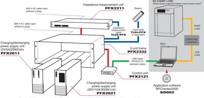
Signal cable: Use a twisted pair cable. This cable is not included in the product package and should be procured by the user.
