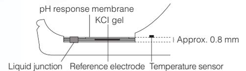
● **Sectional drawing of tip of Flat sensor.**
