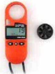
Replacing the impeller restores the PMA-2008 's accuracy.
