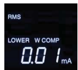
▲AC Hipot (Withstanding voltage) test settings display (example)
