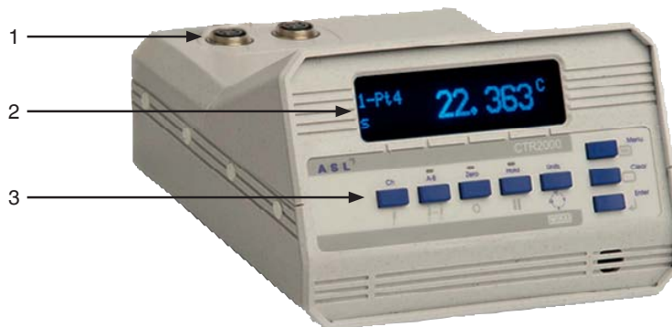
8-Channel precision thermometer, model CTR2000
