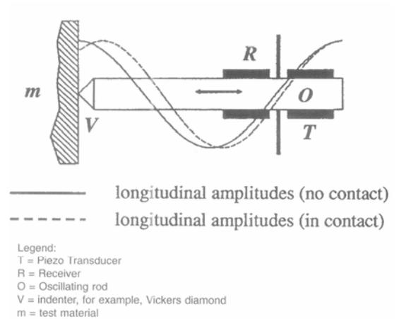
FIG. 1 Schematic Description of the UCI Probe
