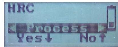
Select the scale. Press the ↓ button. The display will show Test (blinking) Press the Enter the → button to scroll over to “Process” and then press ↓ button to enter ‘processing mode Select your operation by ← or → button and confirm your selection by the ↓ button.
