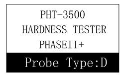
The system will automatically detect the type of the impact device during power up, and would display this information on the screen. Users should pay attention to the probe type displayed on the screen. After pausing for several second, the screen will exit and enter the main display interface.
