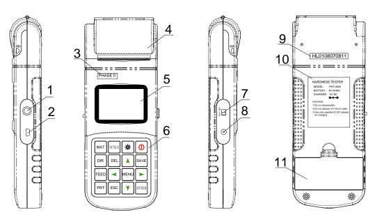
1 Socket of impact device 2 USB port 3 Phase II 4 Paper compartment cover
