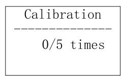
Set the impact direction as [ 1 ]. Measure 5 points on the standard hardness block.
