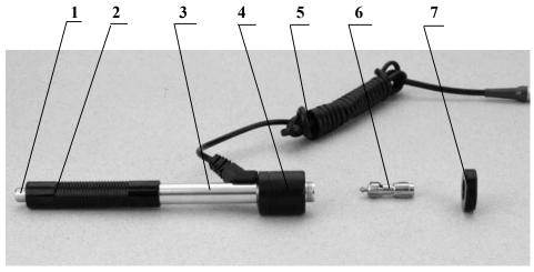
1 Release button 2 Loading tube 3 Guide tube 4 Coil unit
