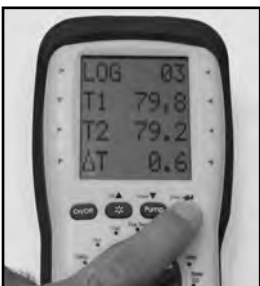
Press and hold "SEND" to log the current readings.
