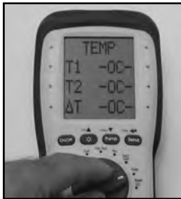
Rotate test selector to Temp
