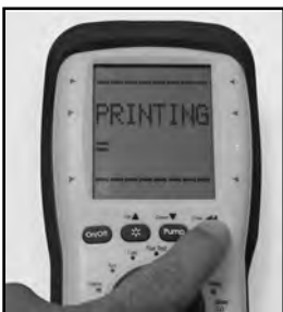
Press "SEND" to start the printout of results from any test screen.
