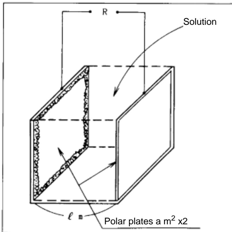
**Fig. 1 Conductivity cell example**
