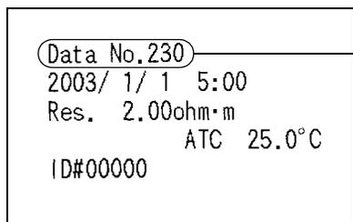
Printer output for Resistivity measurement mode:
