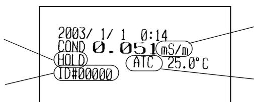
When the data is the data confirmed with Auto Hold, "HOLD" is shown. Nothing is displayed for the instantaneous value measurement.
