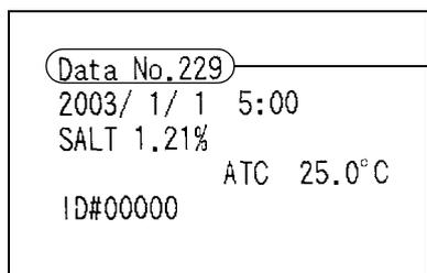
Printer output for Salinity measurement mode:
