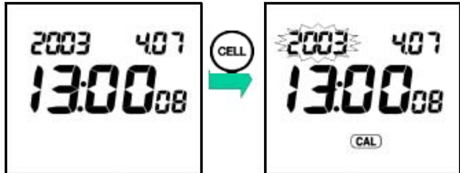
2. Switch the display to year, month, day, hour, minute, and second using the ENTER key. You can set a numerical value using the and keys.
