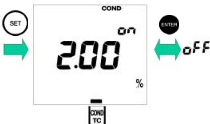
3. Specify a numerical value for the temperature coefficient using the and keys.
