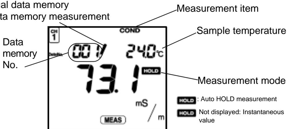
Select and load the desired memory data item using the and keys. The displayed number returns to 0 after 300, the maximum number.
