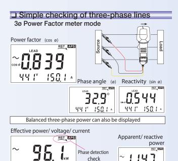
The 3286-20 's three-phase power measurement method calculates and displays the power values for a sine wave input at 50/60 Hz, assuming it is balanced and there is no distortion. Accurate measurement is not possible on a three-phase line if it is not balanced, for example when controlled by an inverter or thyristor.
