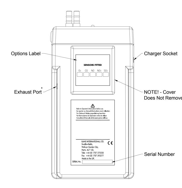
\*NOTE! Do not cover exhaust port as this will severely affect analyser operation
