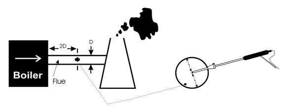
The probe depth stop cone provided with the instrument allows the probe to be used in holes whose diameters range from 8 mm to 21 mm ( $^{5}/_{16}$  to  $^{13}/_{16}$  inch).
