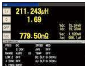
L, Q and Rdc continuous measurement screen
