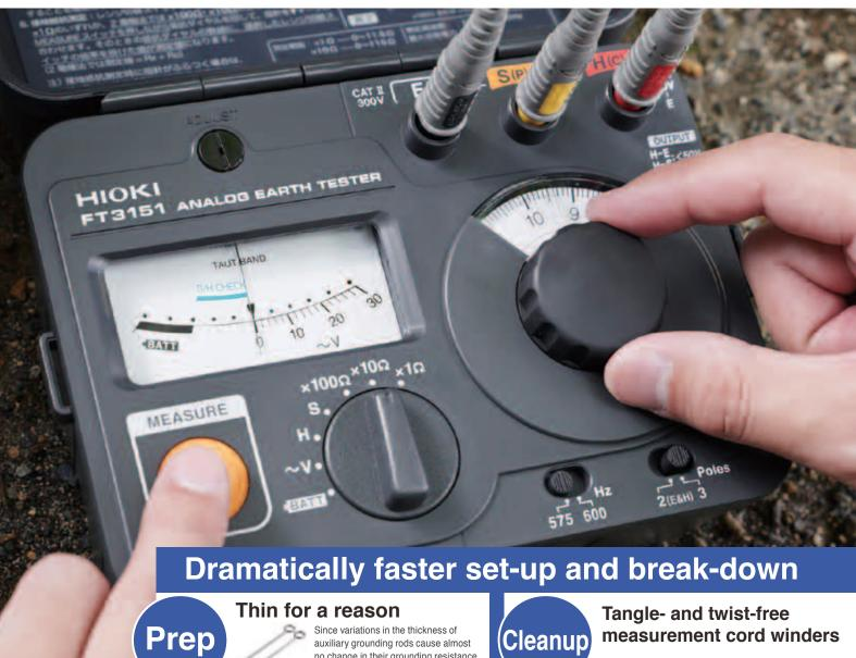
no change in their grounding resistance, the FT3151 uses thinner rods that are easier to drive into the ground
