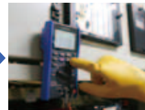
Press the MEM key to save measured values in the instrument's internal memory.
