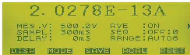
Data display with 0.1 fA resolution (10 pA range).
