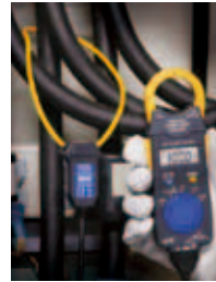
Use with an AC Clamp Meter to measure large wires and currents.
