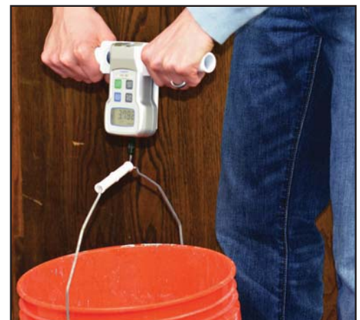
Digital force gauge (100 or 200 lb.) shown with attachable handle. 500 lb. models handles thread into body of gauge
