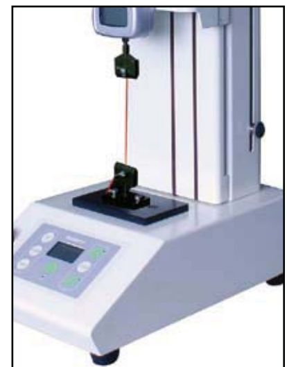
Stand with Optional Grip Performing Tension Test
