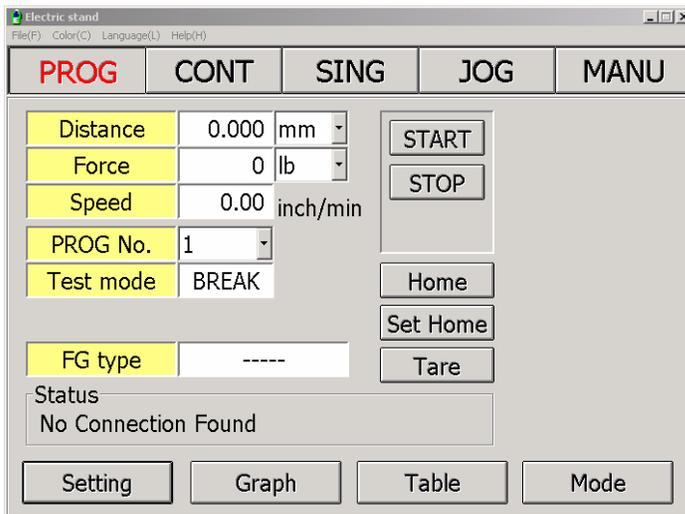
Break is designed for one cycle test, an optional continuance of the test if no break is detected is possible by turning off the return position option.
