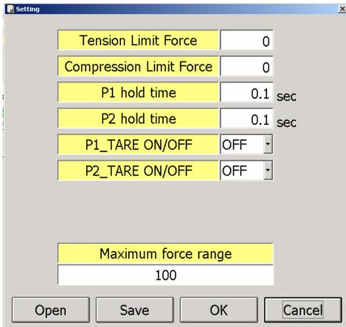
Settings window for single mode allows additional functions such as Tare function both for P1 and P2, P1 and P2 hold time or dwell time
