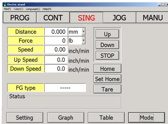
This test performs one complete set for both compression and tension test. Speeds for UP and Down Direction are entered from the main window.
