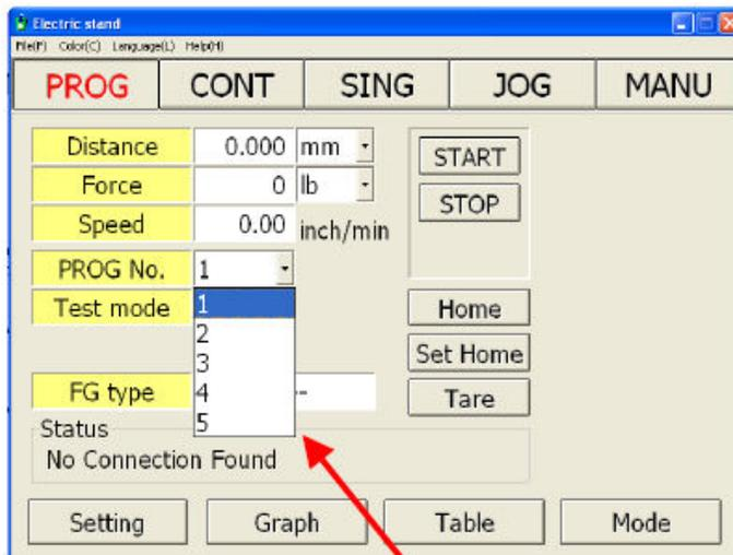
Five different settings can be uploaded for easy testing.
