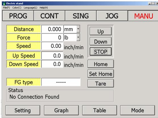
Speed can be adjusted from the main window. Enter value on the UP and Down entry box.
