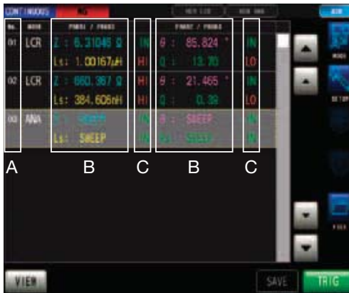
A: Panel numbers set for continuous measurement; B: Measured values; C: Parameter judgment results
