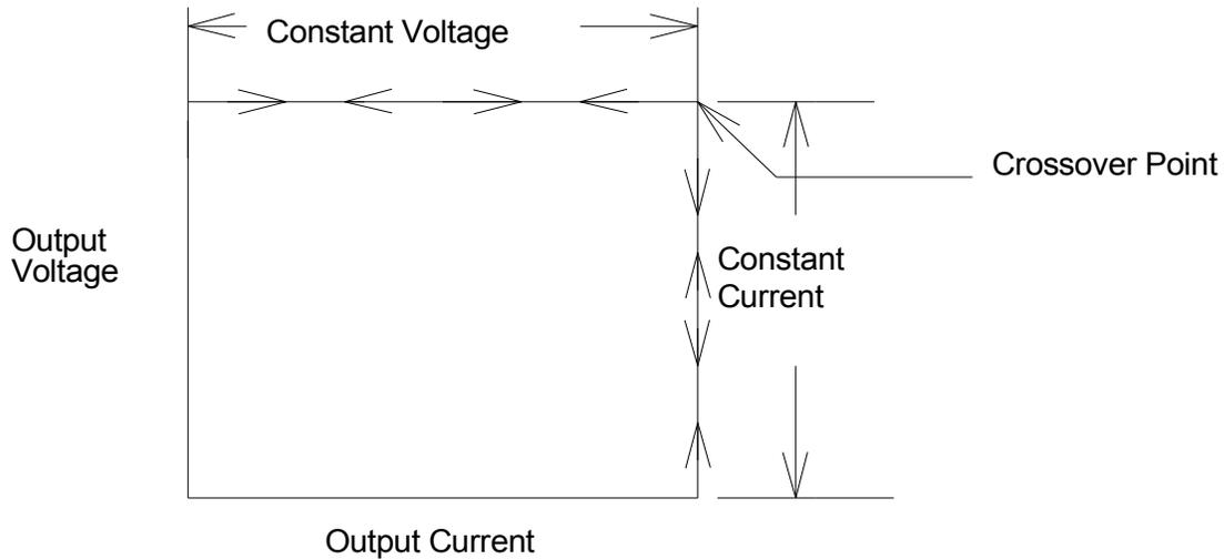
Figure 3 Constant Voltage vs. Constant Current Relation Diagram
