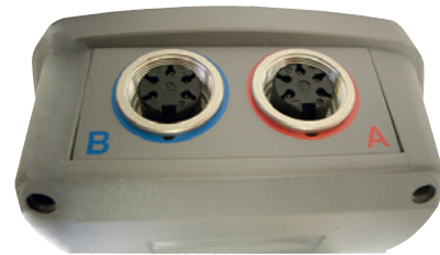
2 Connection port for temperature probe inputs
