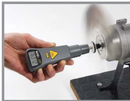
• Contact Tip RPM Measurement
