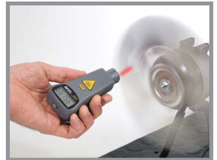
• Non-contact IR RPM Measurement
