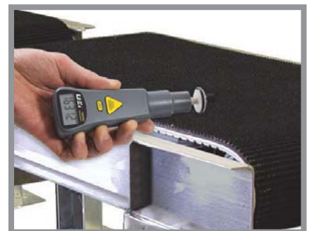
• Contact Wheel RPM Measurement
