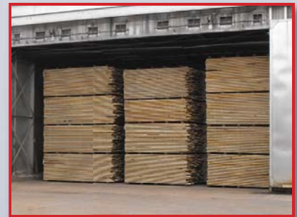
Hardwood boards entering a kiln that will dry them to a moisture content of less than 10%
