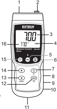
**Notes:** Items 8, 9, and 10 are located behind the snap-off compartment cover on meter's right side. Battery compartment, tilt stand, and tripod mount are located on the rear of the instrument
