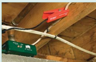
The compact, clamp-style probe accessory can be used on wires that are hard to isolate or reach, or where the RT30 transmitter cannot fit.
