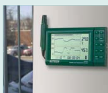
Wall mounted for storage and easy viewing of Temperature and Humidity trends with date/time stamp
