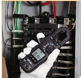
Accu-Tip enables more accurate amperage measurements
