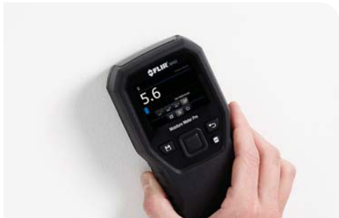
Verify moisture with pinless measurements
