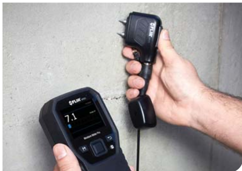
External pin probe for resistive moisture readings
