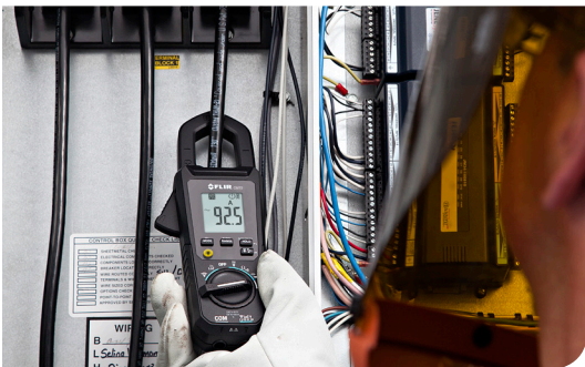
True RMS AC Current up to 600A
