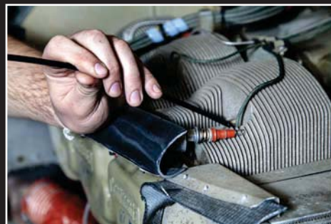
Inspecting cylinder in aircraft motor with VSA2-1M
