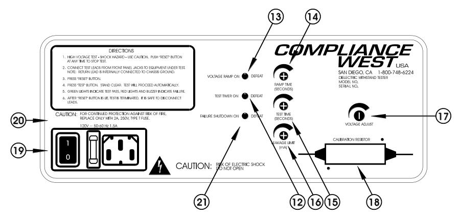
Figure 3-3. Controls, Indicators, Connectors - HT-10000P dc & HT-10000P ac Rear Panel
