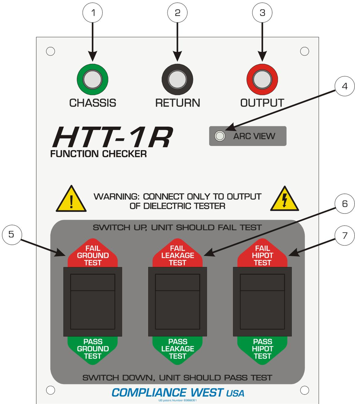
Figure 1: HTT-1R Front Panel Features
