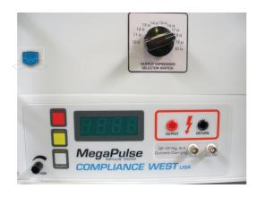
AAMI DF-1 Fig. B.2 waveform Tester with 15 ohm output impedance
