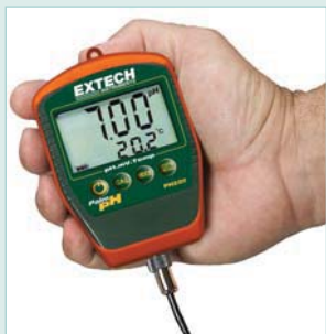
PH220-C includes pH electrode with 39" (1m) cable
