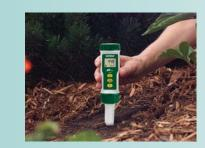
Rugged waterproof (IP57) housing with Flat Surface Electrode for measuring pH in liquids, semi-solids, and solids. Does not break or get junctions clogged like traditional glass bulb electrodes. Easy to replace sensor is perfect for field or lab use.
