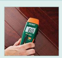
Measures relative moisture of various building materials including wood, particle board, carpeting, and ceiling/bathroom tiles using non-invasive Pinless Technology
