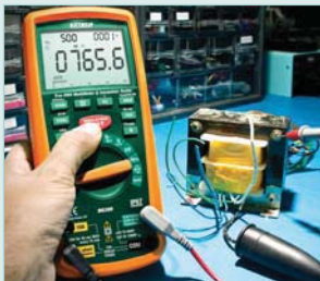
Measure the insulation resistance of transformer windings
